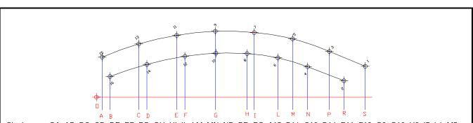
Si misurano:OA, AB, BC, CD, DE, EF, FG, GH, HI, IL, LM, MN, NP, PR, RS, A15, B16, C13, D14, E11, F12, G9, G10, H8, I7, L6, M5, N4, P3, R2 e S1.
